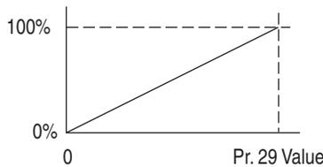
By default, **Parameter 29 - [N2 Ref Scale]** equals 32,767, which is the maximum Reference value for PowerFlex 70/700 drives. Note that additional scaling is performed in the PowerFlex 70/700 drive, where 32,767 equals the frequency selected in drive **Parameter 55 - [Maximum Freq]**. For other DPI hosts, refer to the documentation of the specific DPI host product.
