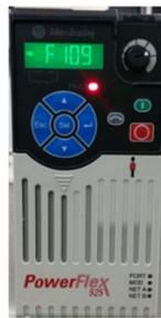
The Control and Power Module are now ready to be configured for compatibility and the fault can be cleared.
